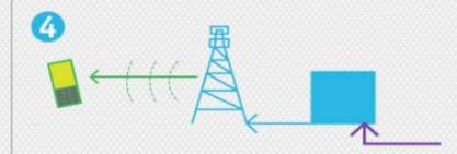
The call (along with many others) gets routed to a backhaul — usually down to an underground wired T1 or T3 line, but sometimes back up the mast to a powerful line-of-sight wireless microwave antenna (typically only used either when there isn't a ground connection, or when the ground connection is poor).
